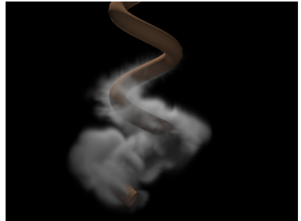
Figure 1: A jet of smoke follows the curve of a helix as it rises ( 60 \times 180 \times 60 fluid grid). The fluid velocities obey slip constraints at the boundaries of the helix, and the smoke is still free to diffuse.
