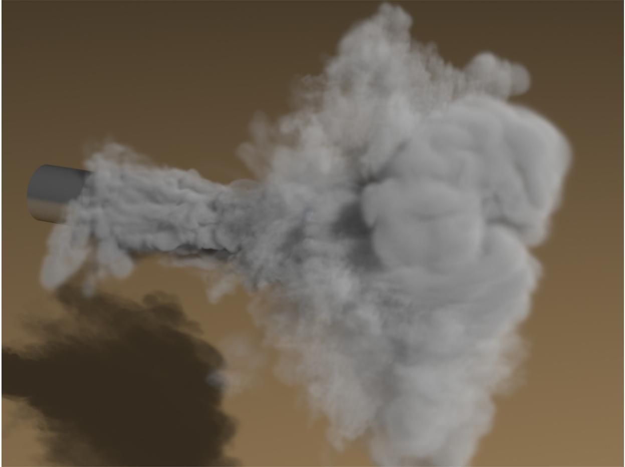
Figure 38: The passive scalar rendered as smoke at  $t = 9.8333$  for the three dimensional smoke jet past rotating ellipsoid example.
